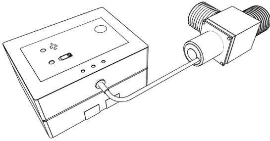
All systems are built with an in-line leak detector. The location may vary depending on placement of the unit. Installation should be on the floor in close proximity of the unit. If you hear beeping and the machine is not producing water then this means a leak has been detected and the automatic incoming water shut off has been activated.
