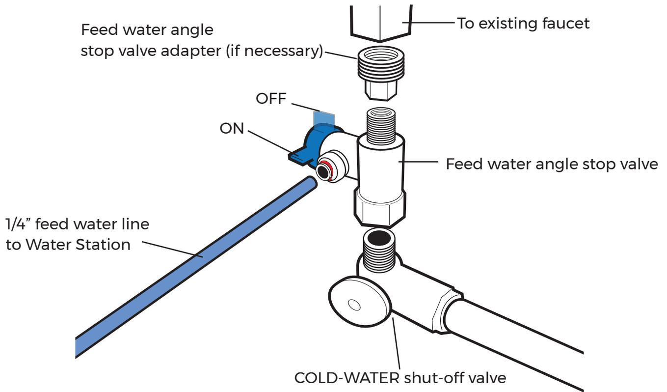
Locate the COLD-WATER Shut-Off Valve underneath the sink and turn it OFF.
