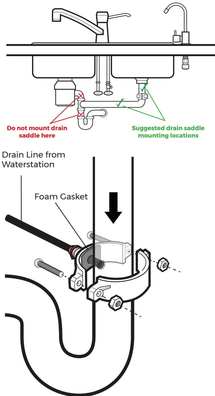
**Never mount drain saddle near garbage disposal to avoid clogging the drain line with debris.**
