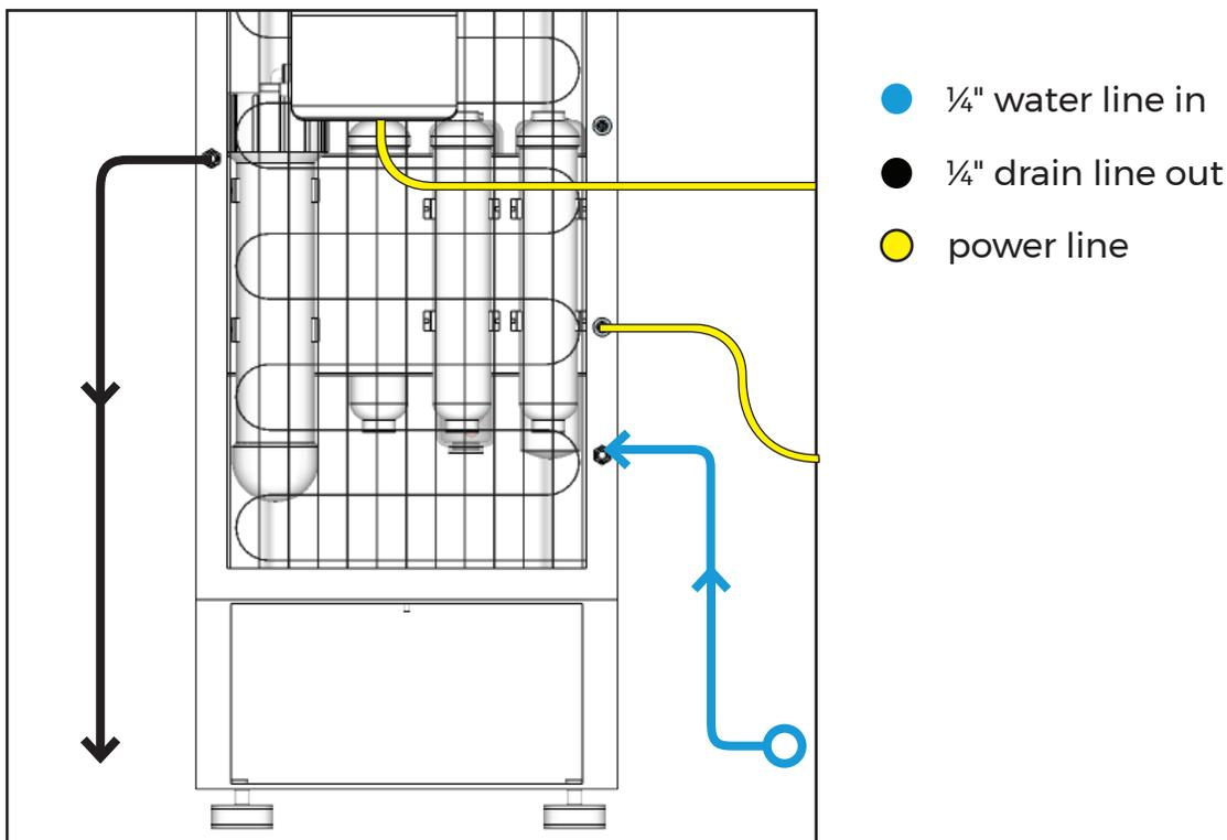
**Please note that a range of incoming water pressure should be no lower than 40 psi and no higher than 70 psi.**
