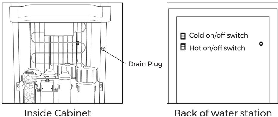
**If unit will not be used for an extended period of time, drain the unit by removing the black drain cap, which is located behind the detachable front panel on the right side. Capture water with a 5 gallon bucket.**
